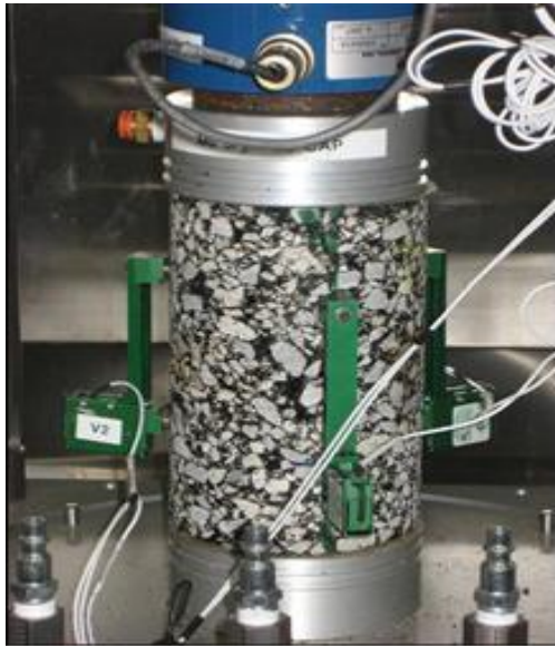
Fig.7. Sensor Configuration for Dynamic Modulus Testing
